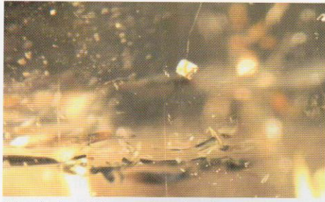
Fig. 4. A solid crystal and other minute solid inclusions in jeremejevite. Transmitted light. 30 x.
