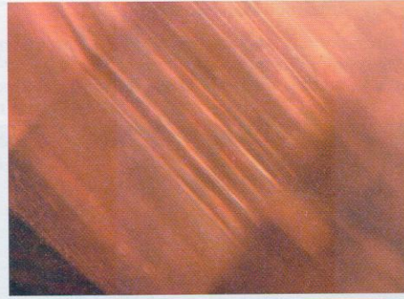
Fig. 3 Parallel tube like inclusions in orthoclase. Dark field illumination, 25x magnification.
